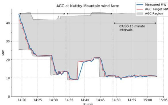
Nuttby Mountain was added to NSPI's AGC dispatch controller for a 45-minute test run. AGC performance was calculated using CAISO and MISO methods.
