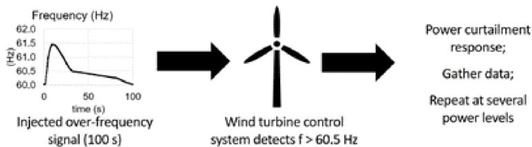
An artificial frequency signal was injected into the control system of one turbine for 39 test runs. A response in proportion to the frequency deviation is expected.
