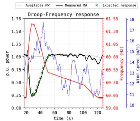
The turbine generators respond as expected, curtailing power (black) in response to the injected frequency (red).
